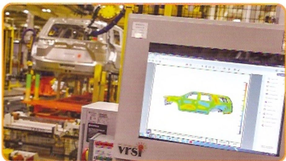
To check for quality, manufacturers might use robotic laser scanners to make a highly detailed color map of the vehicle.
