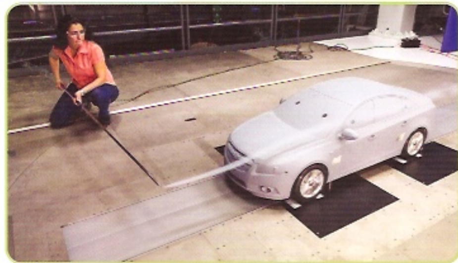
An engineer at General Motors tests a car model in a wind tunnel.
